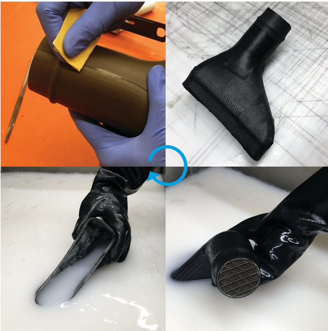
Figure 3 - Sacrificial tools require little prep work and can be used in conjunction with standard composite lay-up procedures. The tool is then dissolved in a detergent solution, leaving the final composite part.
